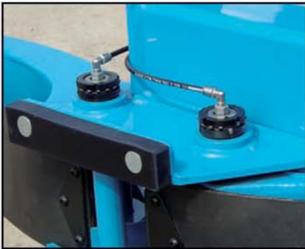
McNeilus grease zerks, heat-treated gears and tapered roller bearings drastically extend the life of replacement arm
